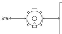
Maintain a minimum distance of 3 meters (10ft.) from overhead construction, walls, rails or other structures.
