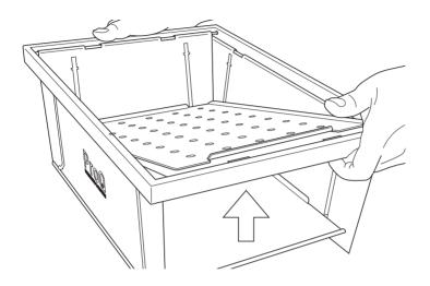
3. Tip the ash out into a suitable non-flammable container.
